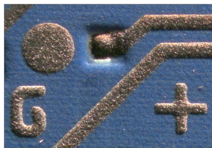
PCB: Laterally grazing reflected light Objective: Plan S 1.0x Magnification 16x (when looking through eyepieces)
